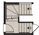
MAIN FLOOR STAIR FOR SECONDARY SUITE
